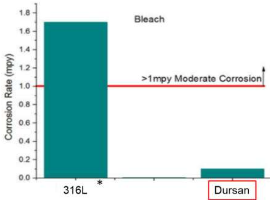
Figure 13 15% (w/w) bleach treatment analysis (SilcoTek Corporation, 2020b). * The substrate was tested by SilcoTek Corporation for other manufacturing environments, but not related to or proposed in this CPS project.
